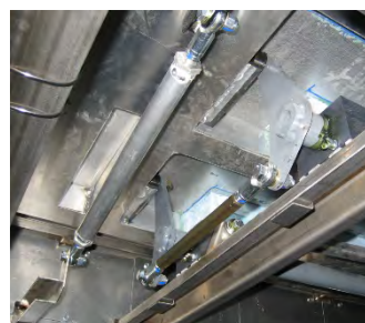
Flat-floor support and lifting mechanism
